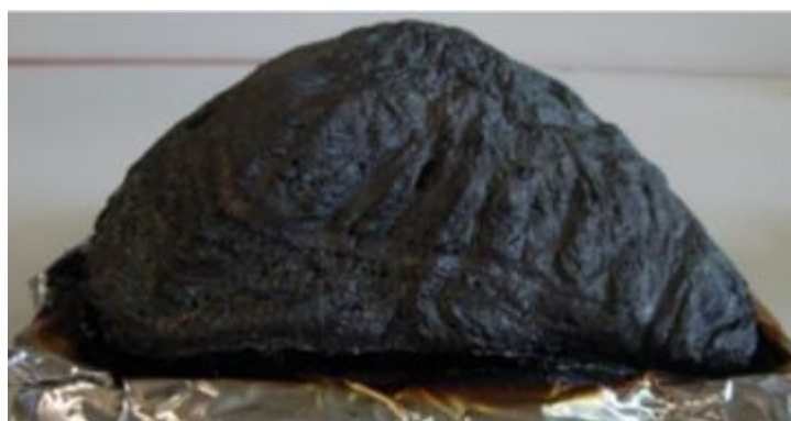
Figure 5 : Example of an intumescent expanded char
