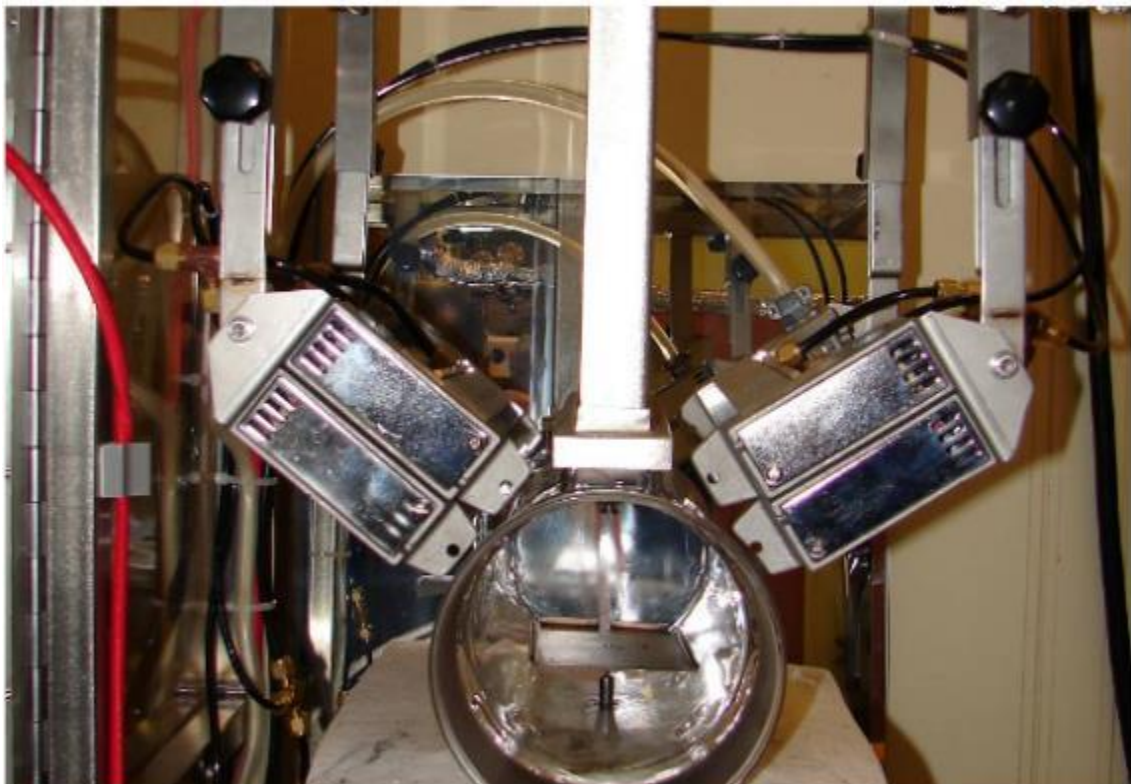
Figure 16: Picture of the radiant furnace used for ASTM E1678/NFPA 269 test (Source: NIST)
