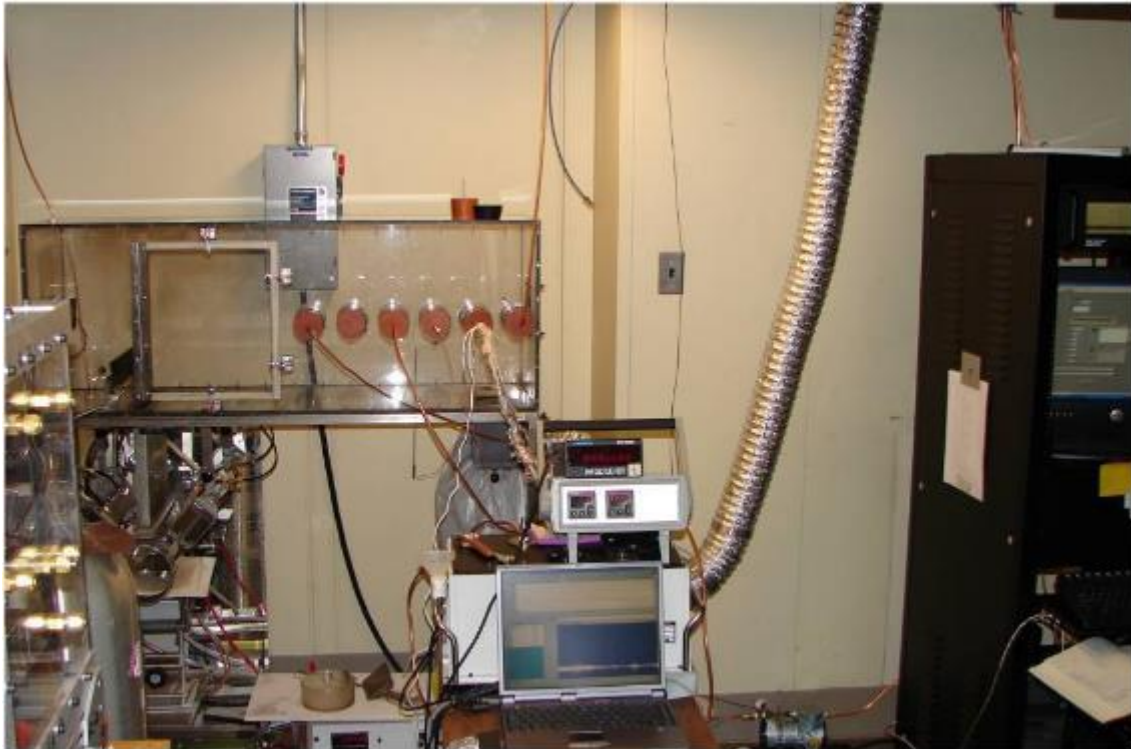
Figure 15 : Picture of the ASTM E1678/NFPA 269 test apparatus (Source: NIST)
