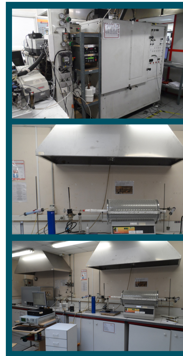
Images: smoke toxicity chambers and tubular furnaces used by Crepim.
