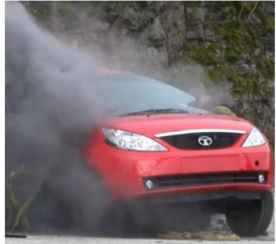
Figure 4 Test 1 – The photo is taken 2 min after the drop, and large amount of smoke are produced from the battery
