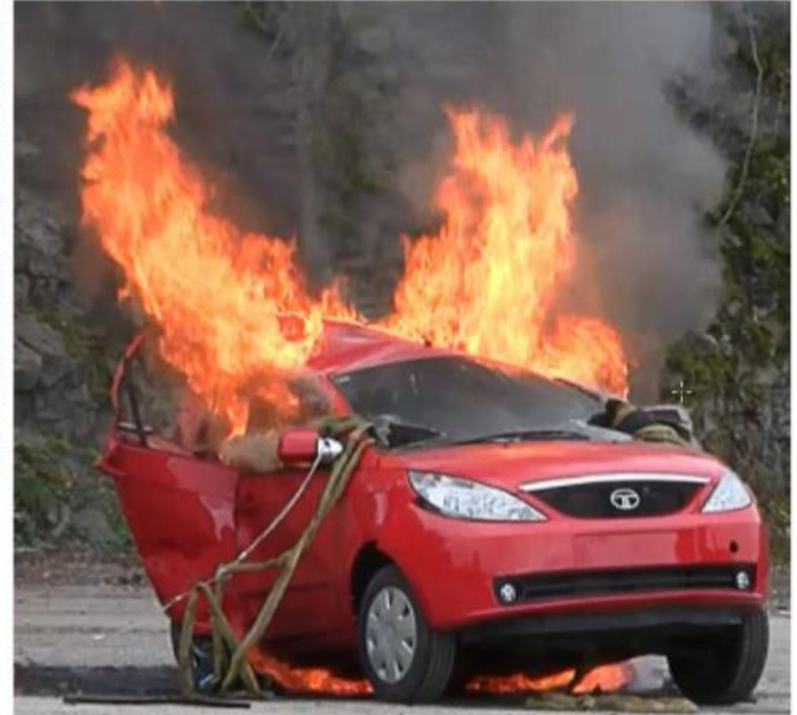
Figure 5 Test 1 – The photo is taken 8 minutes after the drop. At this point the car has started to burn vigorously.
