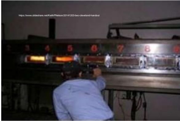
UL 723 “Steiner tunnel test”
