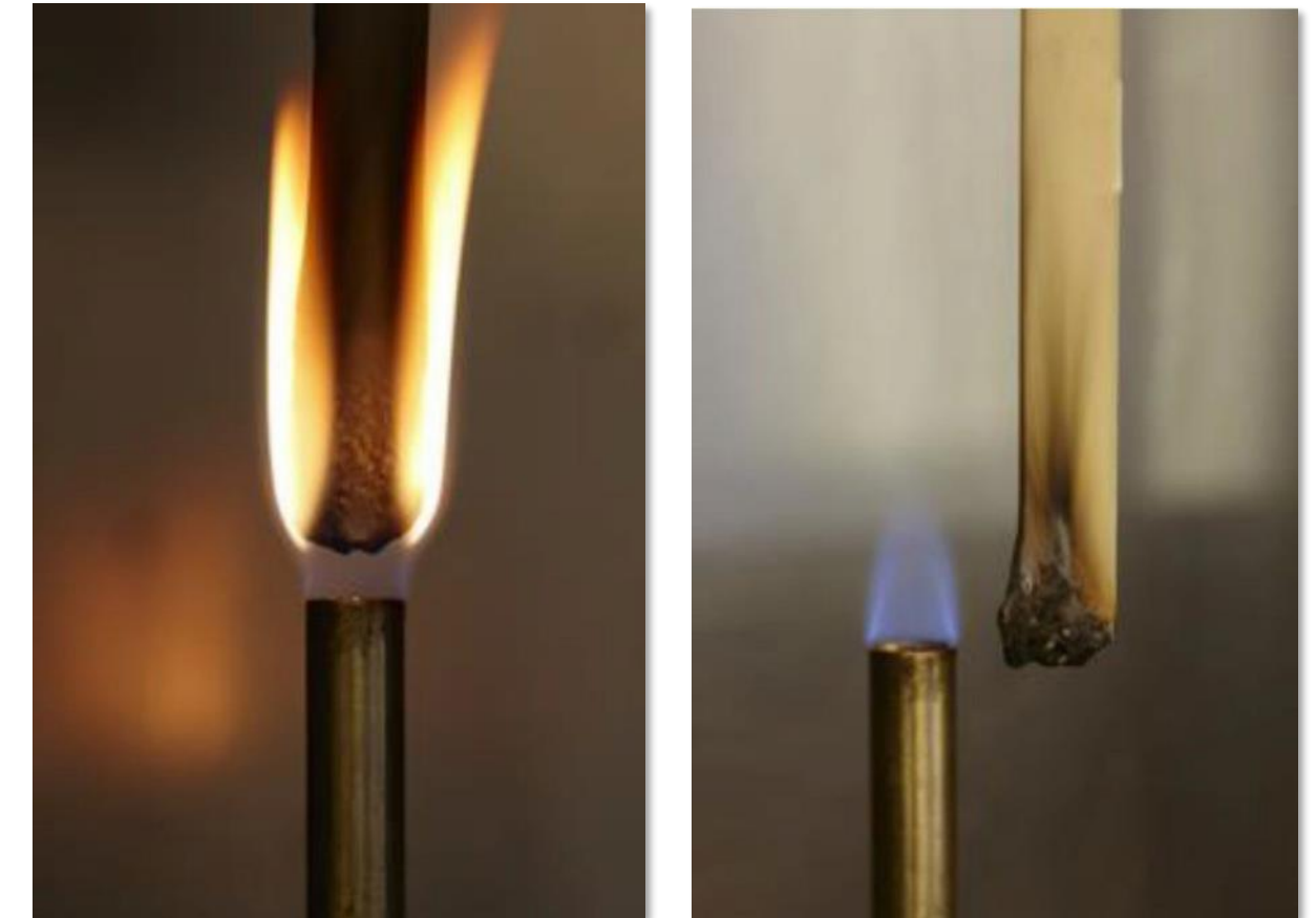
UL 94 vertical fire test. Simulates resistance against ignition by a small flame.
