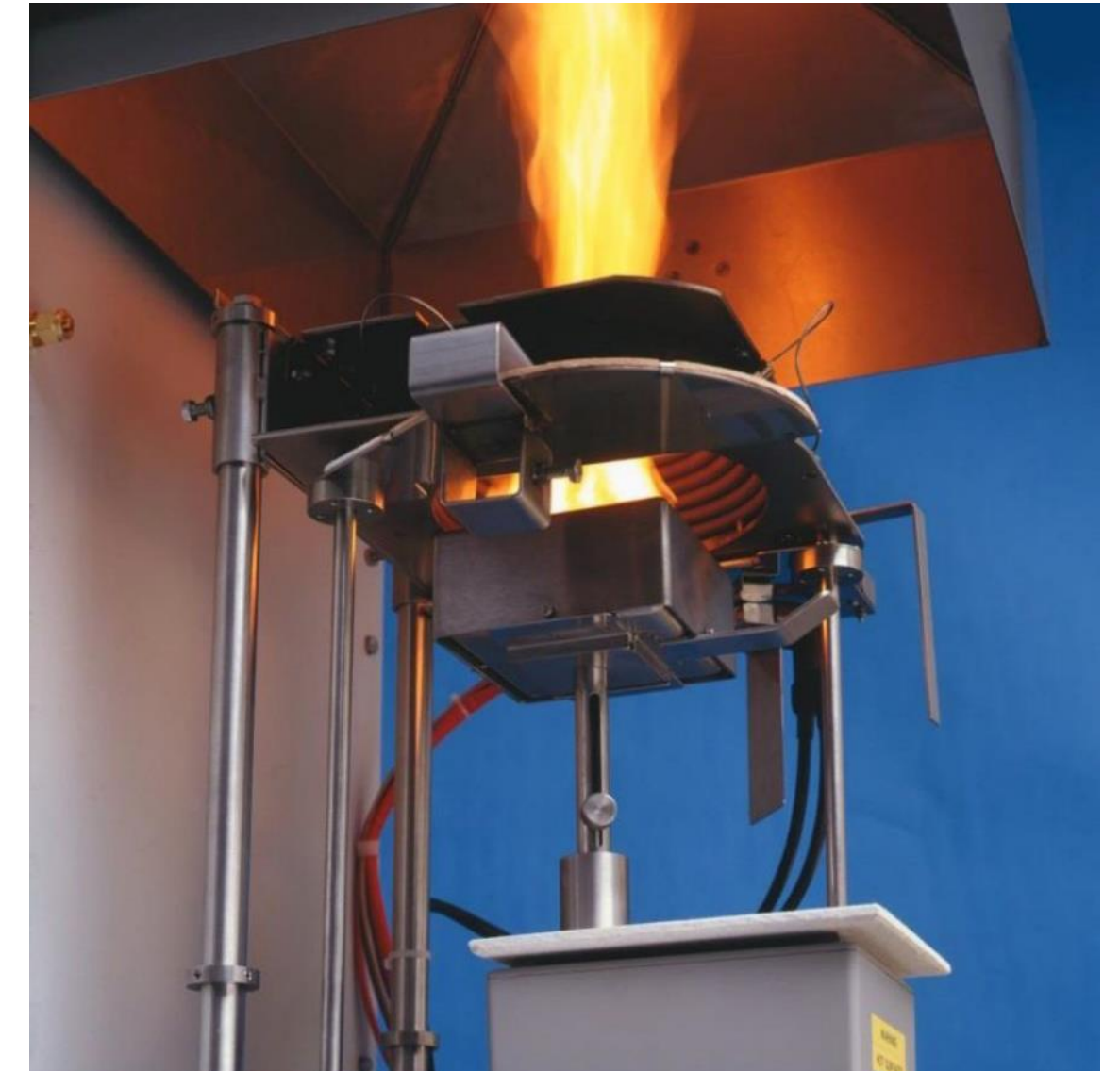
Cone calorimeter fire test. Photos courtesy of Fire Testing Technology, UK
