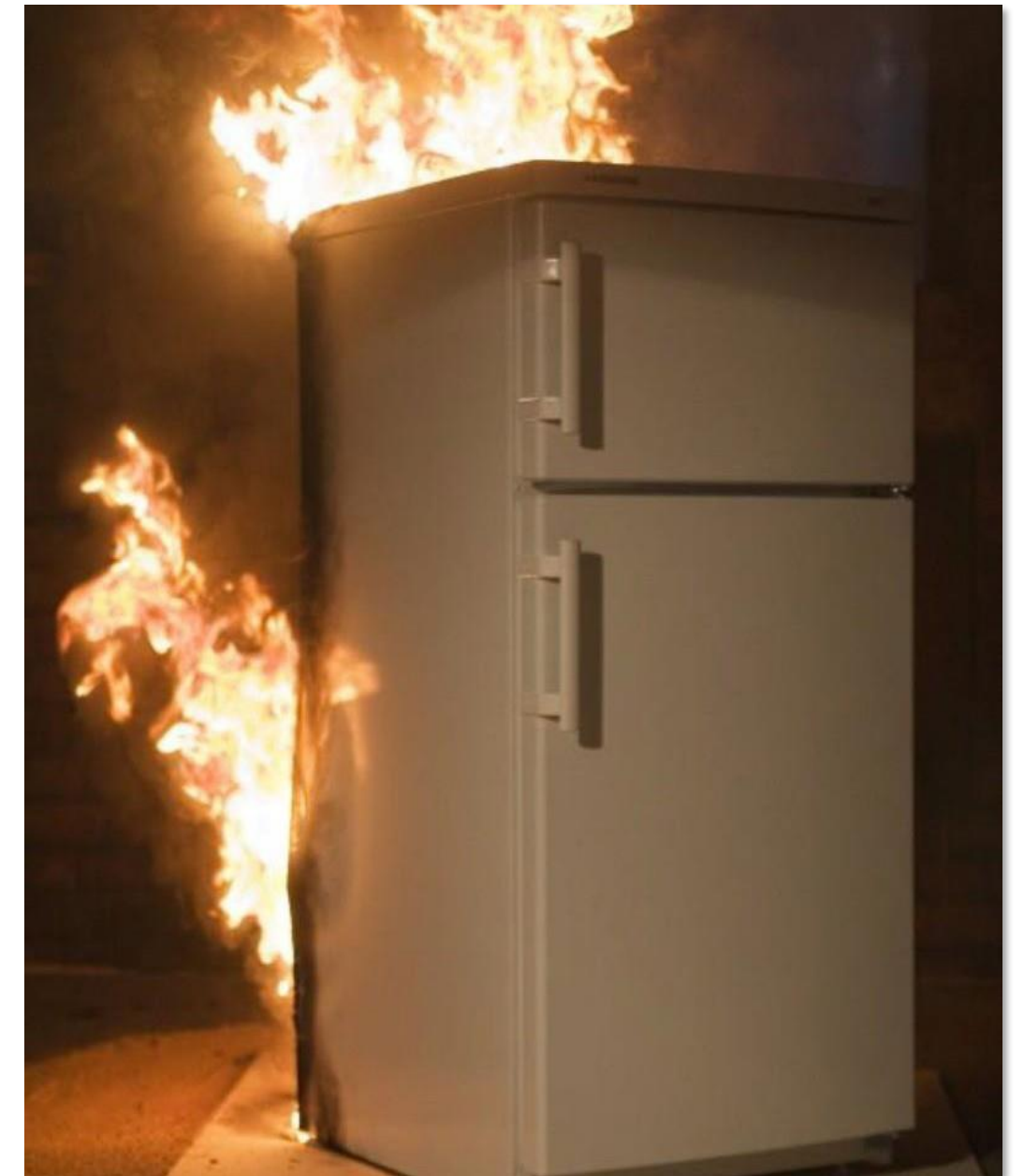
Fire test of a generic fridge freezer.
