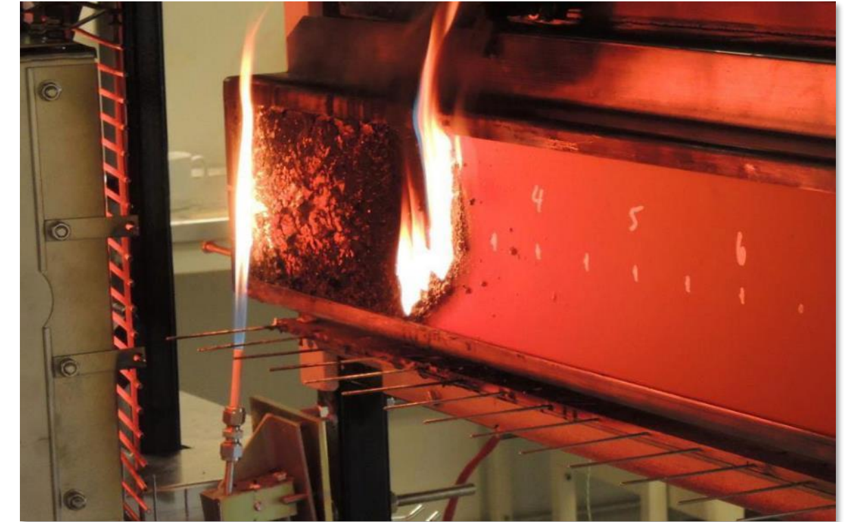
ISO 5658-2 lateral flame spread fire test. Photo © RiSe .
