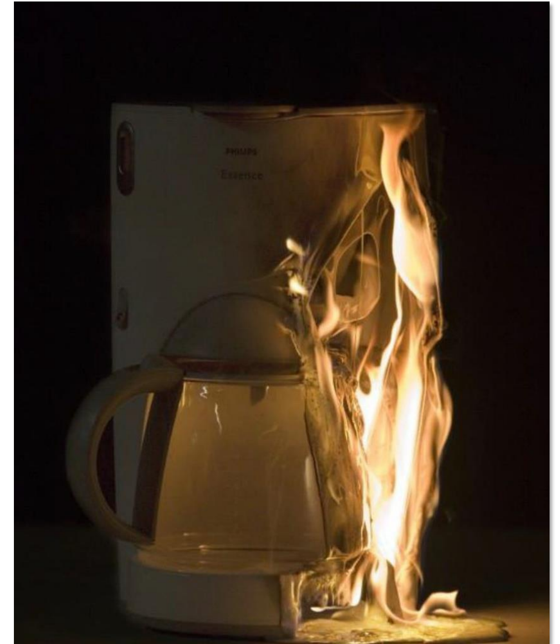
Coffee machines like this one can burn for more than 30 min. Photo © EFRA, Ralf Baumgarte
