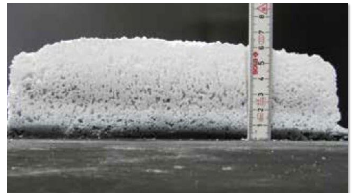
PIN intumescent coatings protect flammable materials, timber, steel or concrete from fire, Photos: © Clariant
