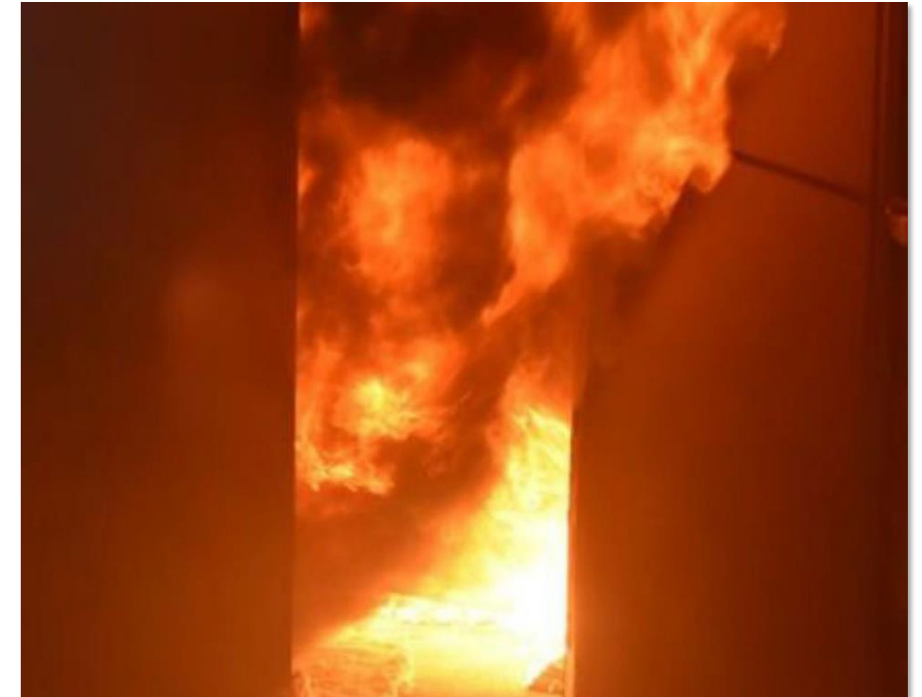
Photo from Blais et al. 2019 https://doi.org/10.1007/s10694-019-00888-8 . Room with non flame retarded contents 8 ½ minutes after start of fire test.
