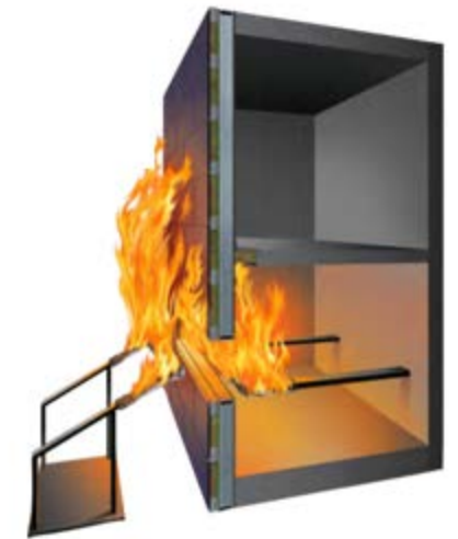
(a) CAN/ULC S134 test (source: glascurtain.ca ) (b) NFPA 285 test (source: thermafiber.com )
