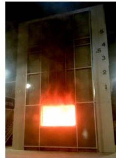
(a) CAN/ULC S134 test (source: glascurtain.ca ) (b) NFPA 285 test (source: thermafiber.com )
