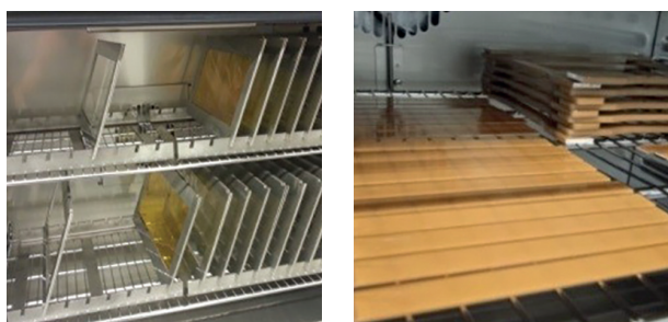
Accelerated oven ageing of specimens, reprocessed granules, as subsequently extruded into films or injection molded into specimens
