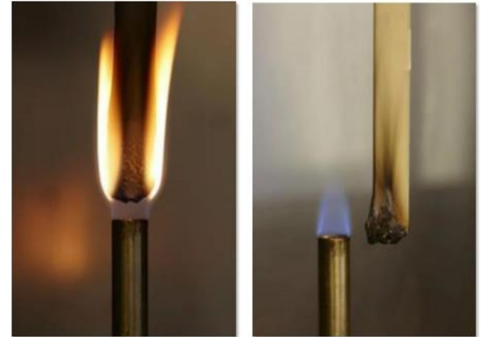
UL 94 vertical fire test. Simulates resistance against ignition by a small flame. Photos © Clariant R. Baumgarten
