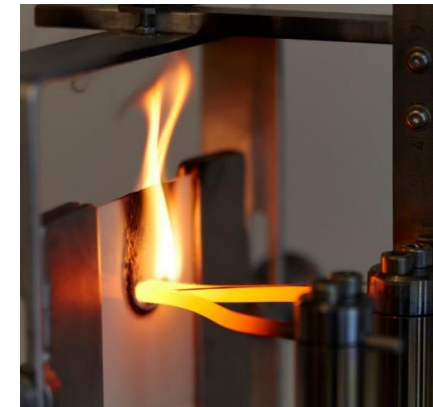
Glow wire fire test. Used widely for electrical and electronic equipment. Simulates resistance to ignition or fire spread from a localised, high temperature heat source, comparable to electrical faults
