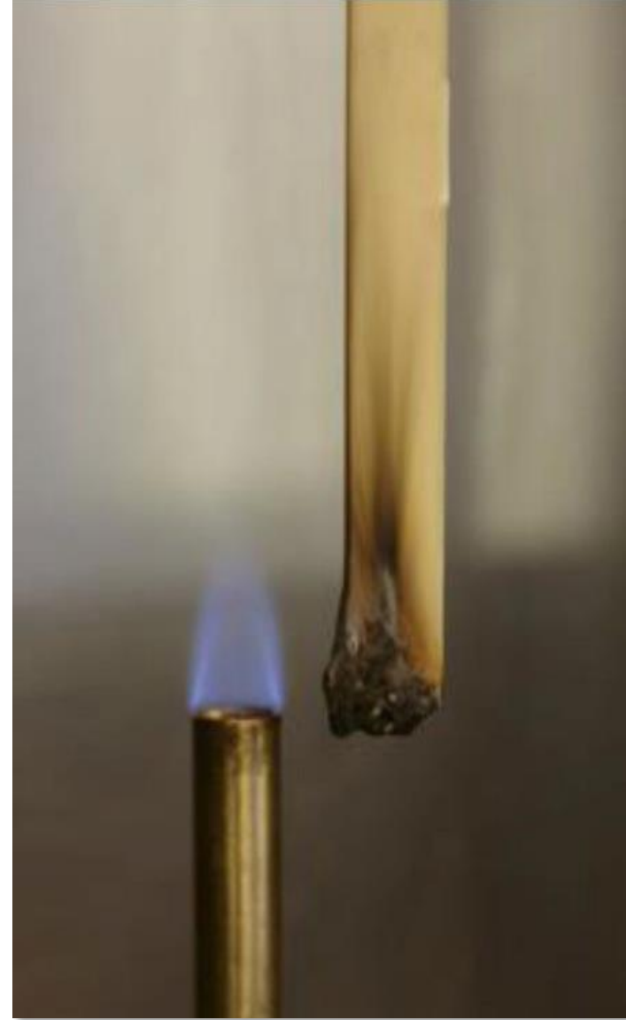
UL 94 vertical fire test. Simulates resistance against ignition by a small flame. Photos © Clariant R. Baumgarten
