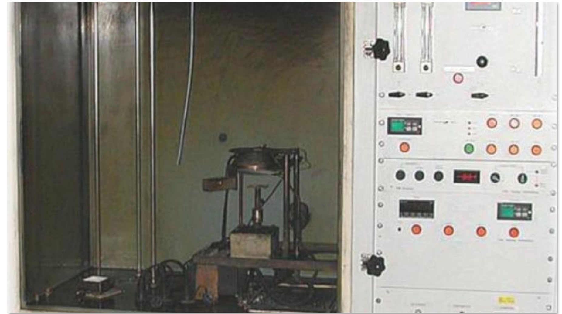
Smoke chamber ISO 5659. Photo © courtesy of Crepim
